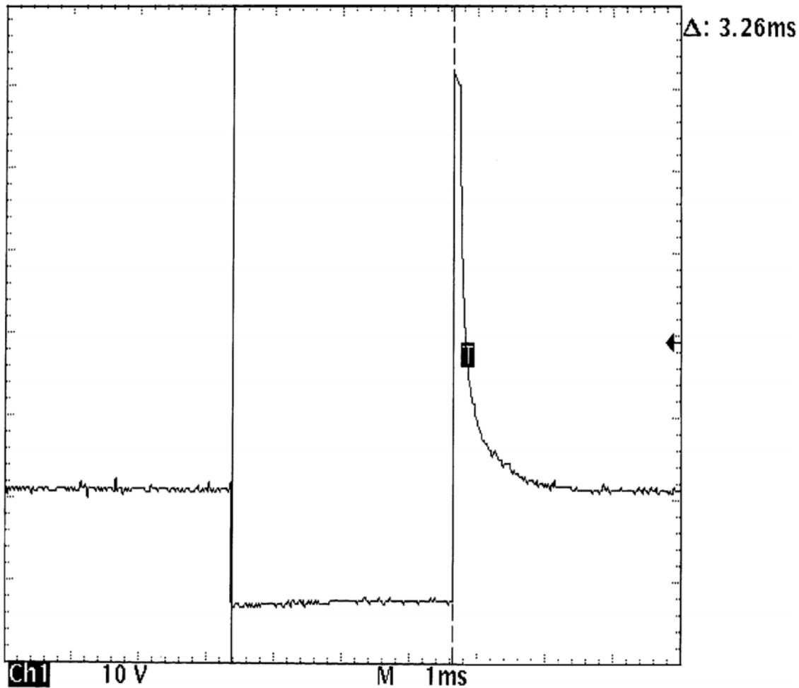
**Fig. 19: Injector Bank - Known Good - Voltage Pattern**
