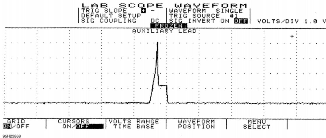
**Fig. 13: Injector Bank w/Normal Current Flow - Current Pattern**
