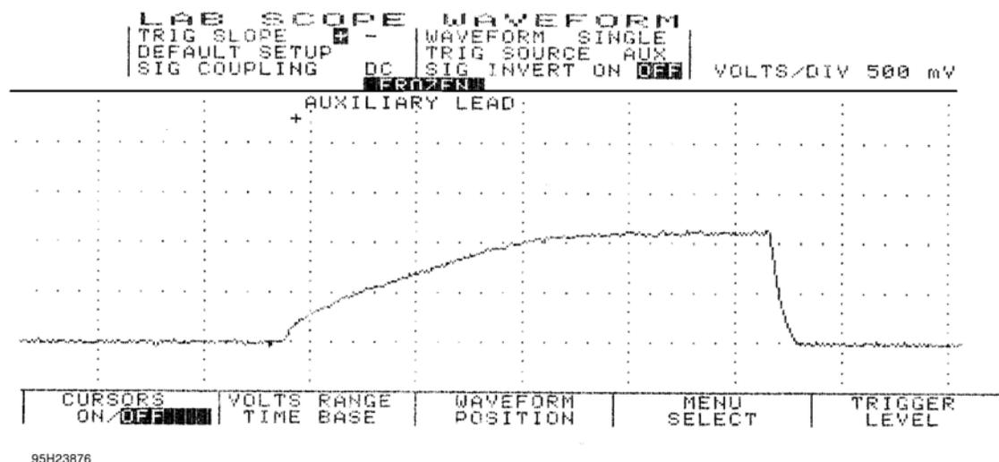
**Fig. 11: Single Injector w/Excessive Current Flow - Current Pattern**
