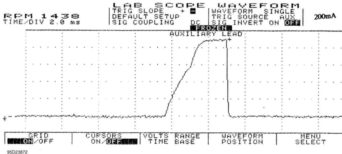
**Fig. 12: Single Injector w/Normal Current Flow - Current Pattern**
