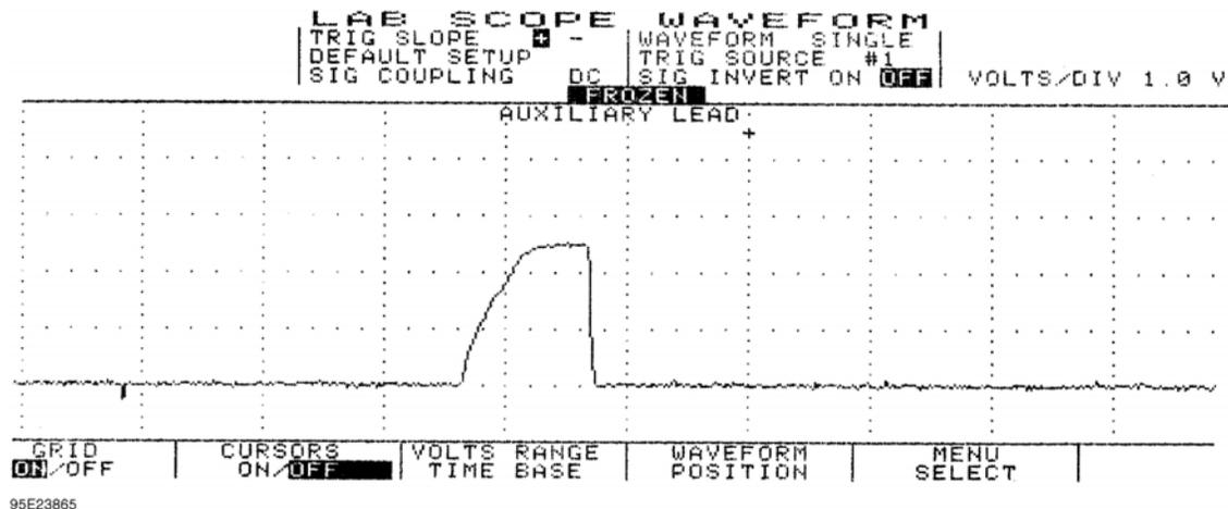
**Fig. 5: Injector Bank w/Excessive Current Flow - Current Pattern**
