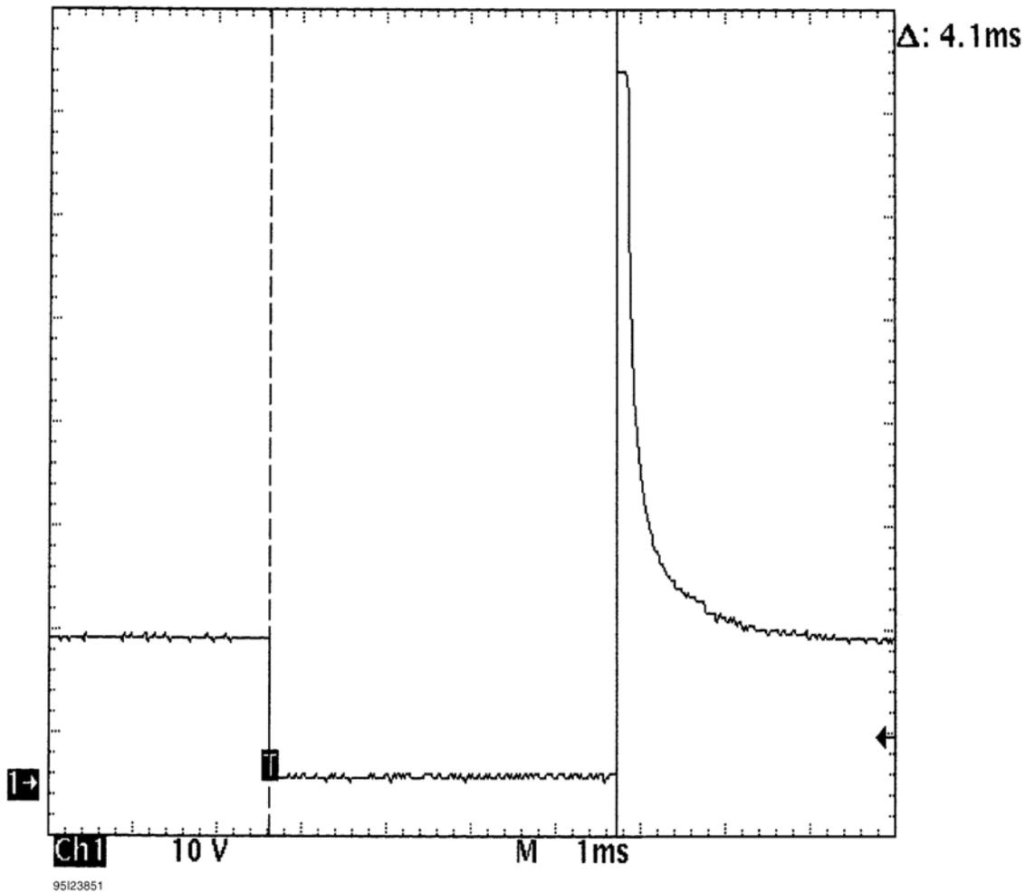
**Fig. 20: Injector Bank - Known Good - Voltage Pattern**
