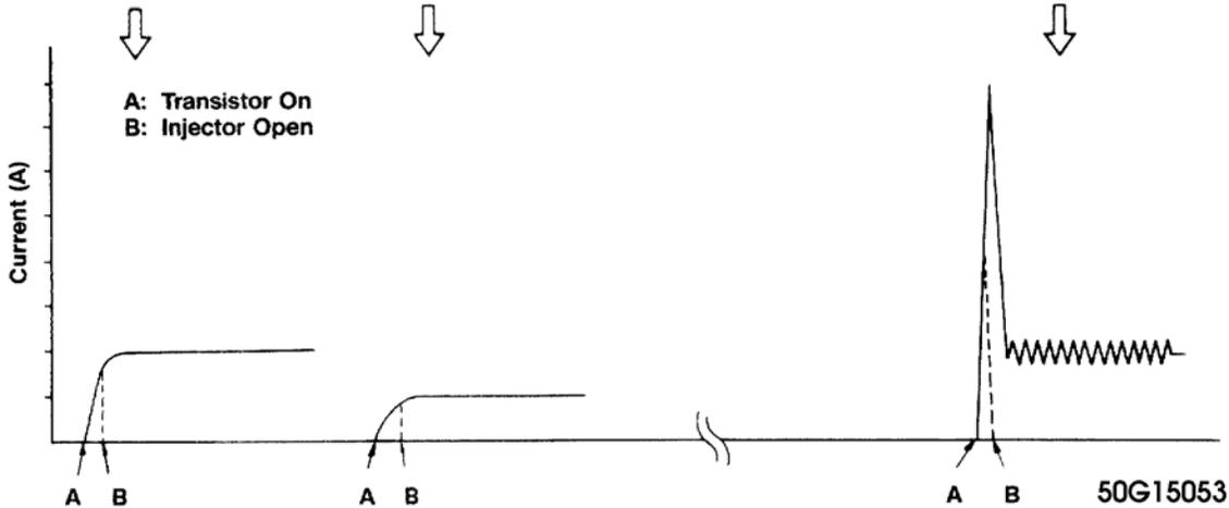
**Fig. 1: Injector Driver Types - Current and Voltage**
