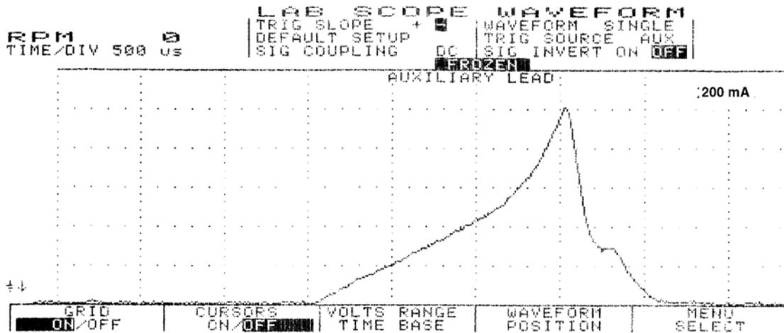
**Fig. 14: Single Injector w/Normal Current Flow - Current Pattern**
