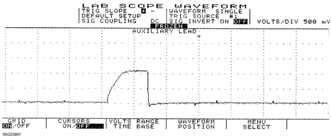
**Fig. 7: Single Injector w/Excessive Current Flow - Current Pattern**
