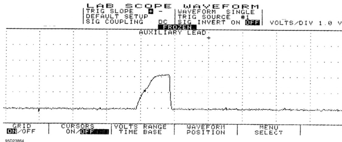
**Fig. 4: Injector Bank w/Normal Current Flow - Current Pattern**
