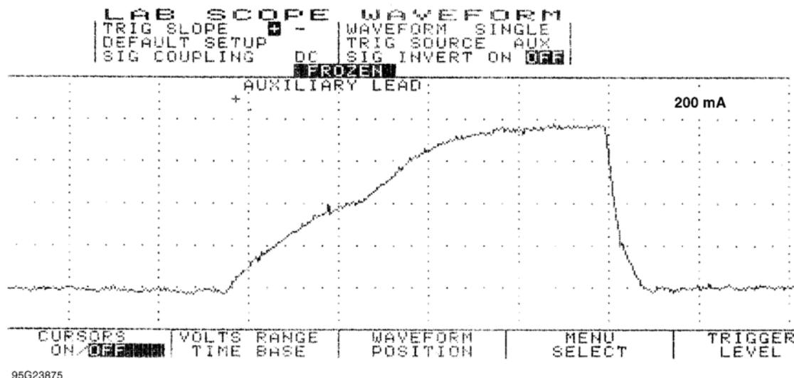
**Fig. 10: Single Injector w/Normal Current Flow - Current Pattern**
