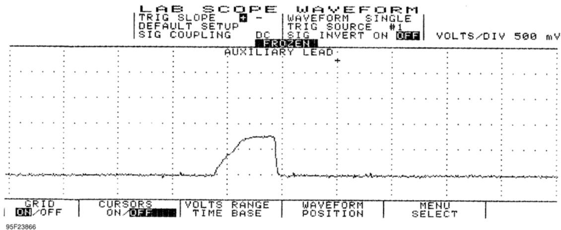
**Fig. 6: Single Injector w/Normal Current Flow - Current Pattern**
